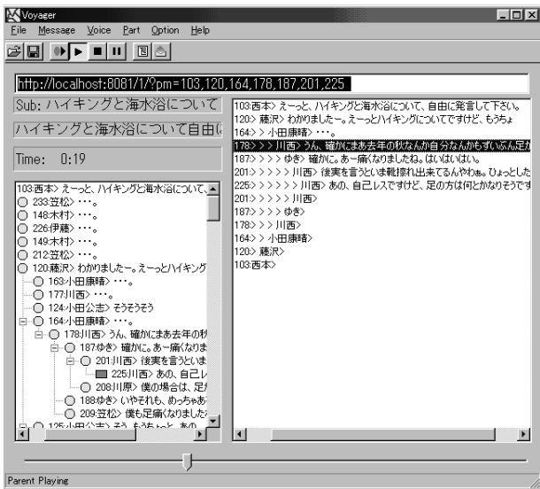
Figure 4: The user-agent software (VOYAGER). Left pane is the tree-view and right pane is the text-view.
